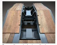
Remove the center bogie section to reveal a V-style boom trough with V-pan for hauling an excavator. The 2-piece lift system makes it easy to convert.
